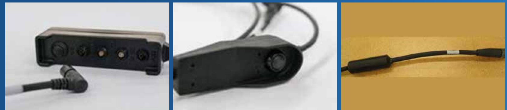
i3 manufactured housing with switch and 4 I/O connectors
